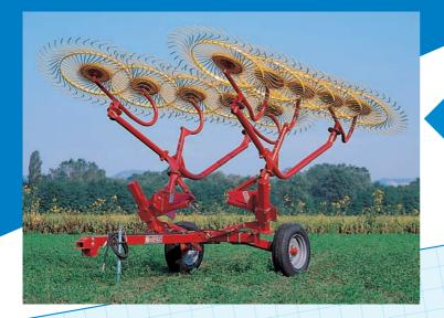
Rake folds into transport position automatically when lifted by means of hydraulic cylinder supplied with the cart. he H/90 V-8-10-12 unit is very simple to use and gives excellent working results.
